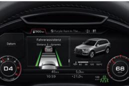
Lane departure warning This feature helps the driver stay in their chosen lane by warning them with steering pulses whenever the lane marking is inadvertently crossed.
