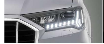
Matrix LED headlamps with dynamic turn indicators\* Precise, high-resolution and perceptive. The Audi Matrix LED headlamps are the right choice to illuminate the road ahead. Besides lighting up your path precisely, the lamps also adjust their beam to avoid dazzling any oncoming vehicles. Their unique design makes them integral not just to the driver, but also to the design language of the car.
