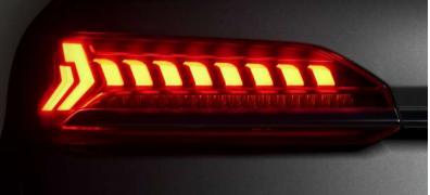
LED rear combination lamps with dynamic turn indicators\* Another must have for your car, the LED rear combination lamps are known for their fast activation, improving visibility for those in the rear. Striking, dynamic LED strips illuminate the rear, segment-wise while making turns, creating a pulse of light that runs outwards in the direction in which the car is turning.
